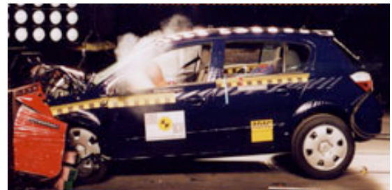
Offset crash test at 64km/h
