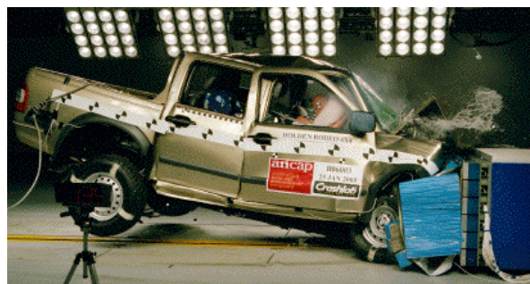
Offset crash test at 64km/h
