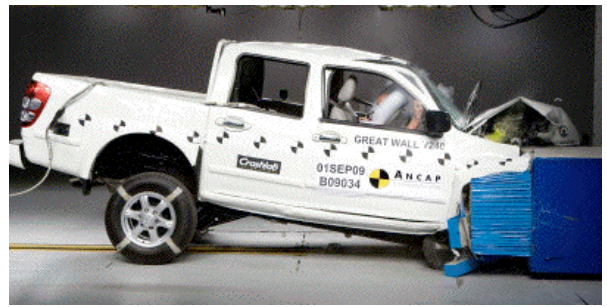
Offset crash test at 64km/h
