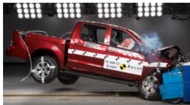
Frontal offset test at 64 km/h
