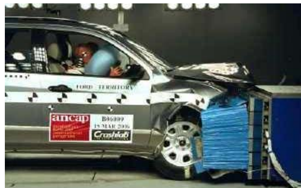
Frontal offset test at 64 km/h
