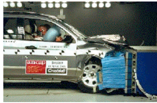
Offset crash test at 64km/h (2006)
