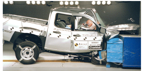
Offset crash test at 64km/h
