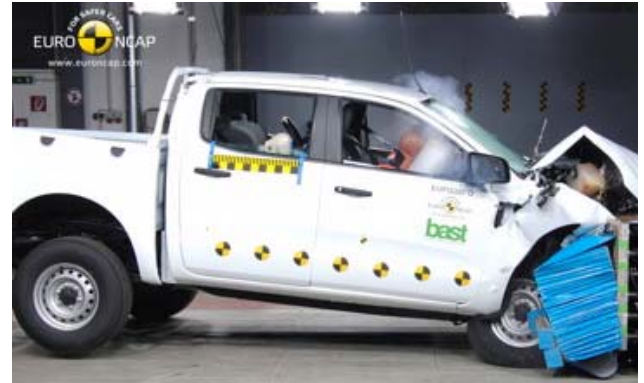
Frontal offset test at 64 km/h (Euro NCAP)
