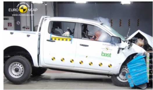
Offset crash test at 64km/h
