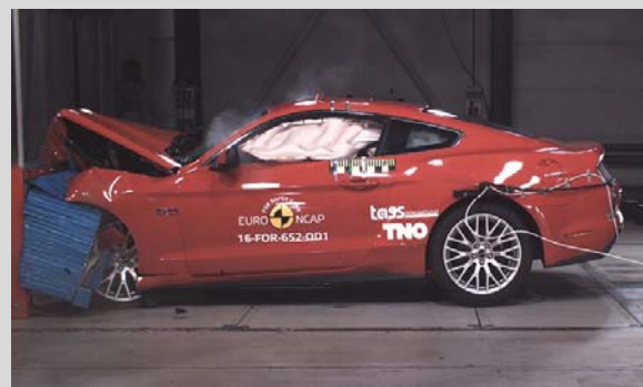
Frontal offset test at 64km/h
