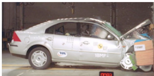
Offset crash test at 64km/h
