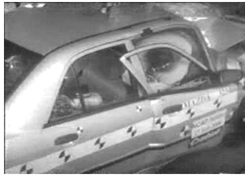
Offset crash test at 64km/h
