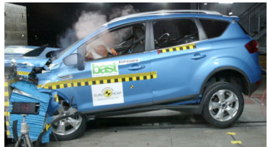
Offset crash test at 64km/h
