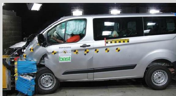
Frontal offset test at 56km/h
