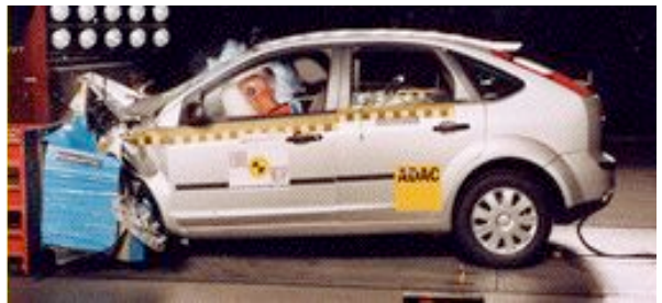
Offset crash test at 64km/h
