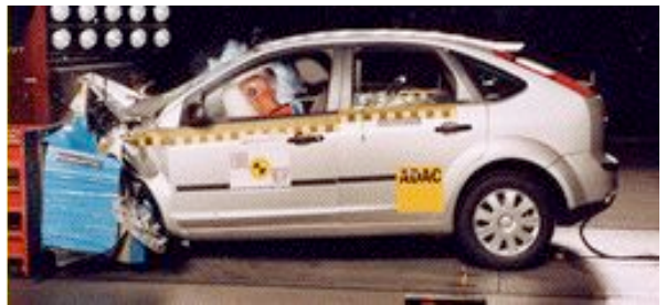
Offset crash test at 64km/h
