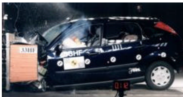
Offset crash test at 64km/h
