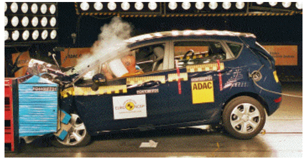
Offset crash test at 64km/h (Fiesta hatch)
