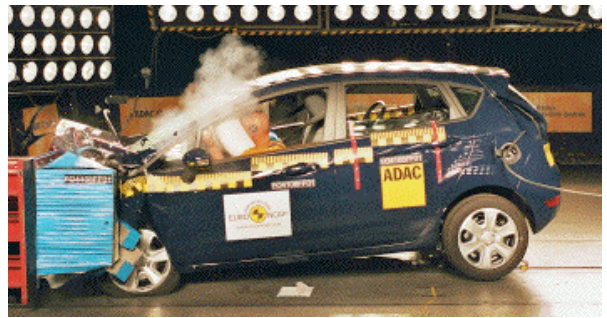
Offset crash test at 64km/h
