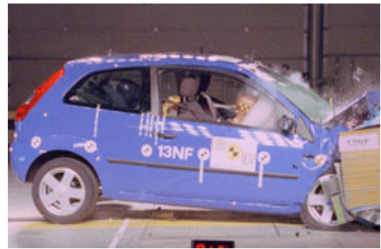
Offset crash test at 64km/h
