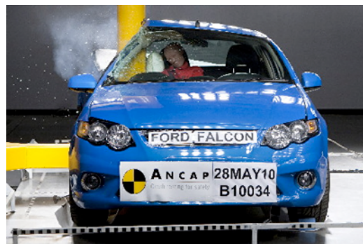
Side pole crash test at 29km/h
