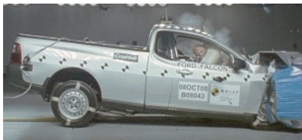
Offset crash test at 64km/h
