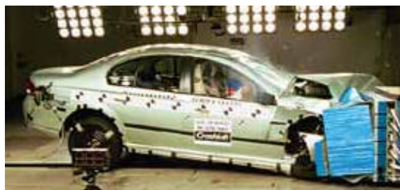
Offset crash test at 64km/h
