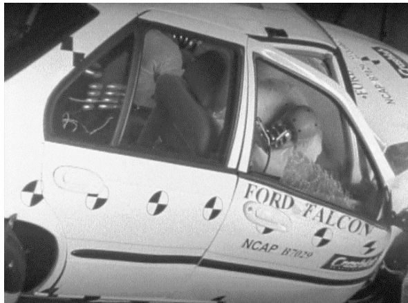
Offset crash test at 64km/h
