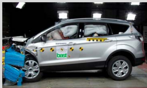
Frontal offset test at 64km/h
