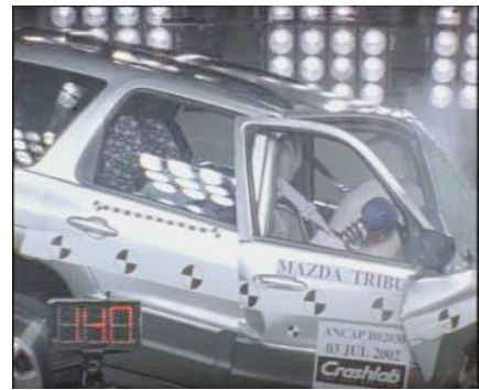
Offset crash test at 64km/h
