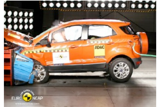
Frontal offset test at 64 km/h (Euro CAP)
