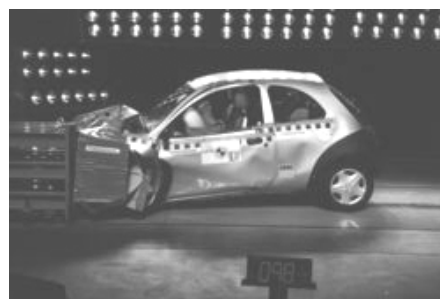
Offset crash test at 64km/h
