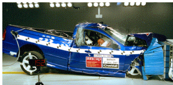
Offset crash test at 64km/h
