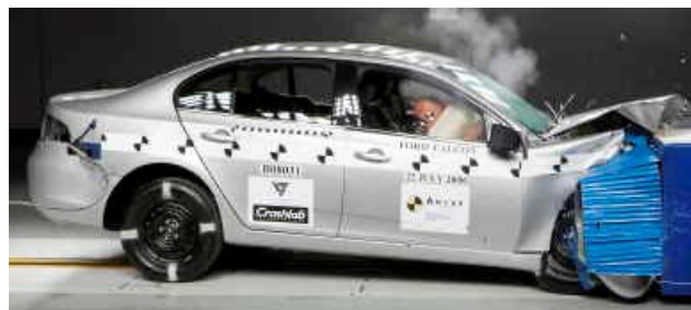
Frontal offset test at 64 km/h
