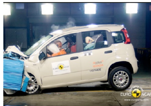
Frontal offset test at 64 km/h (Euro NCAP)
