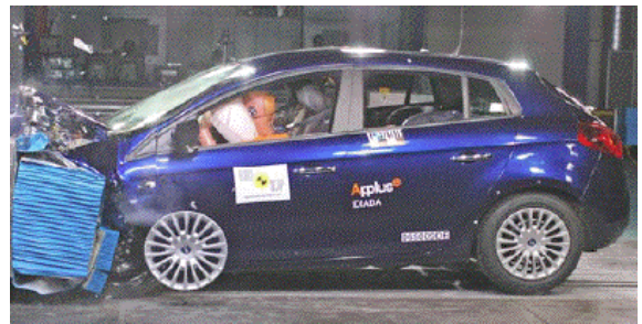
Offset crash test at 64km/h (front hubcap dislodged)
