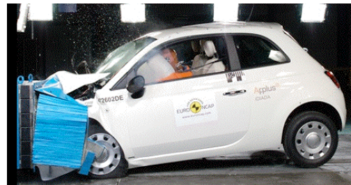
Offset crash test at 64km/h
