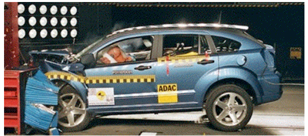
Offset crash test at 64km/h
