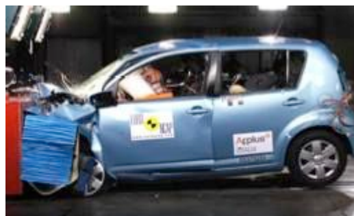
Offset crash test at 64km/h
