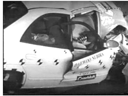
Offset crash test at 64km/h
