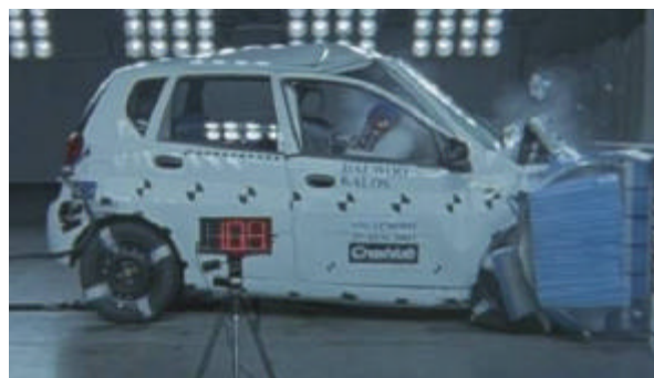
Offset crash test at 64km/h
