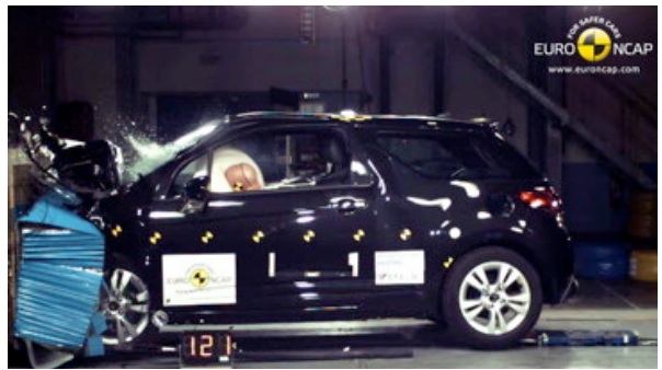
Offset crash test at 64km/h
