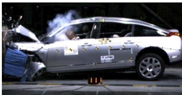
Offset crash test at 64km/h
