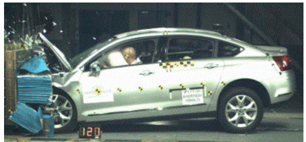
Offset crash test at 64km/h
