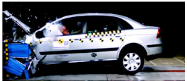
Offset crash test at 64km/h
