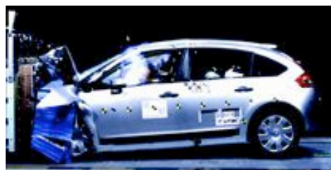
Offset crash test at 64km/h
