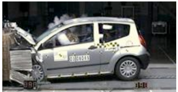
Offset crash test at 64km/h
