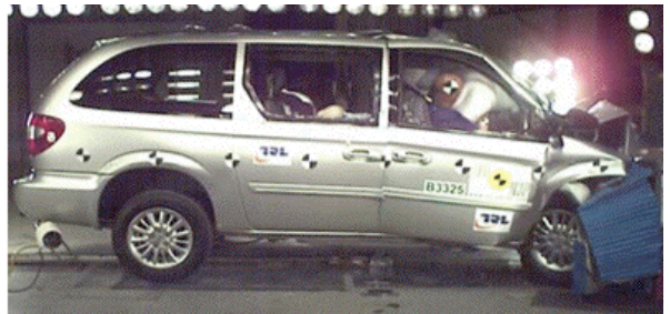
Offset crash test at 64km/h
