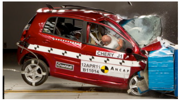
Offset crash test at 64km/h
