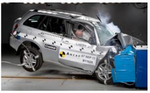
Offset crash test at 64km/h
