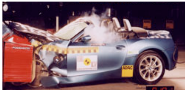
Offset crash test at 64km/h
