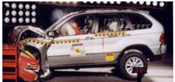
Offset crash test at 64km/h
