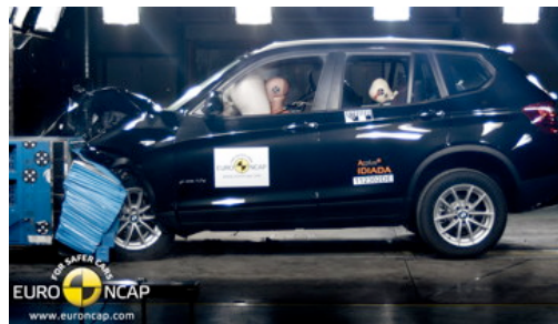
Offset crash test at 64km/h
