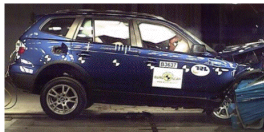
Offset crash test at 64km/h
